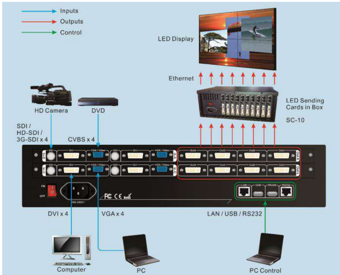
Picture 3-2 hardware connection diagram
